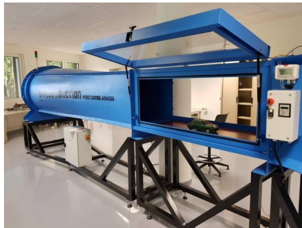
Figure 5.1.1. Wind Tunnel of the ESTACA
